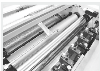
VARNISH APPLICATION UNIT
